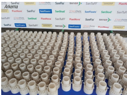
FIGURE 1. Distillation tray bubble caps made from polyvinylidene fluoride (PVDF) resin can be a viable option in cases where metallic components are subject to acid attack
